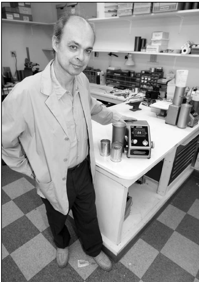
Bill Fraser of Quantum Electronics in Brandon says the digitalized moisture tester with built-in calibration has a digital display that eliminates eye strain and errors in reading.
